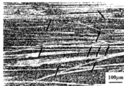
Fig. 12. Scanning electron micrograph taken from the fracture surface of the fiber layer of a single edge notched A-GFML-90 specimen.
